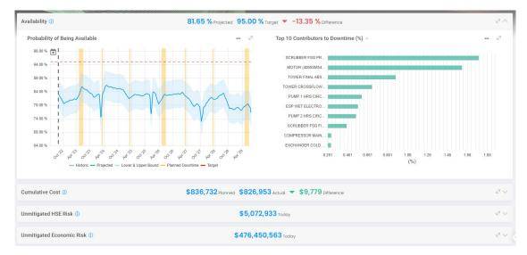
This is an example of the system view based on a facility's current tasks. The facility is currently on track to achieve 81.65% availability based on the current tasks. Additionally, this view is able to identify the top 10 contributors to downtime, with the scrubber and motor ranking as the top two contributing factors to downtime.
