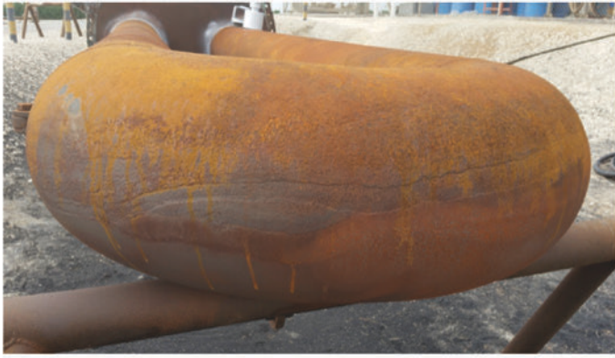
Figure 2. Photos showing creep damage on the firetube of the Glycol Reboiler.
