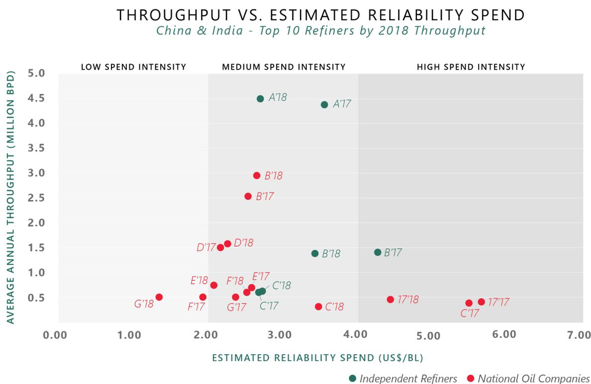
Figure 4. Estimated reliability spend vs. throughput, top 10 refiners in China by 2018 throughput
